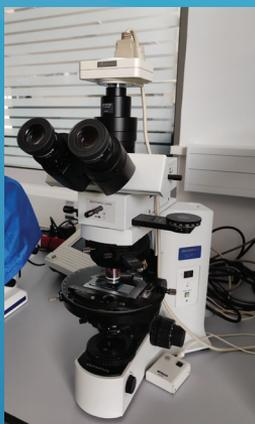
Figure 1. Olympus/Evident polarized light microscope
