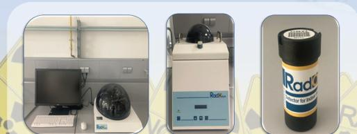
Figure 2. RadoSys- Radon measurement system
