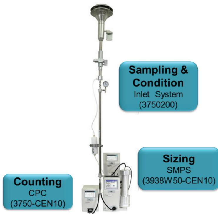
**Figure 1.** CEN-compliant solution for UFP measurements of PSD and PNC including the dedicated sampling system.
